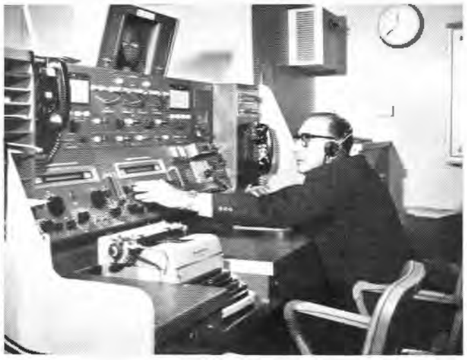
COMMUNICATIONS CENTER —L. B. Victor, Manager of Moore-McCormack's radio and electronics department, makes final check of liner's "communications center." The center, developed by RCA, consists of radiotelegraph and radiotelephone consoles providing radio and phone service from every stateroom to both sides of the Atlantic.
