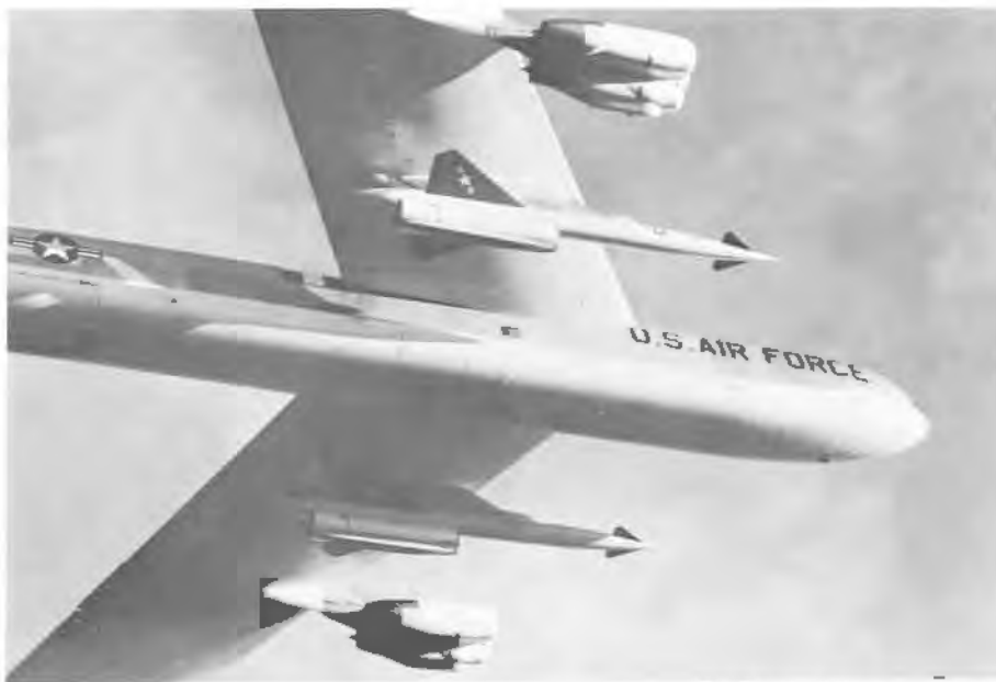
SAC —A Strategic Air Command Boeing B-52 bomber carries a Hound Dog missile under each wing, near the fuselage.
