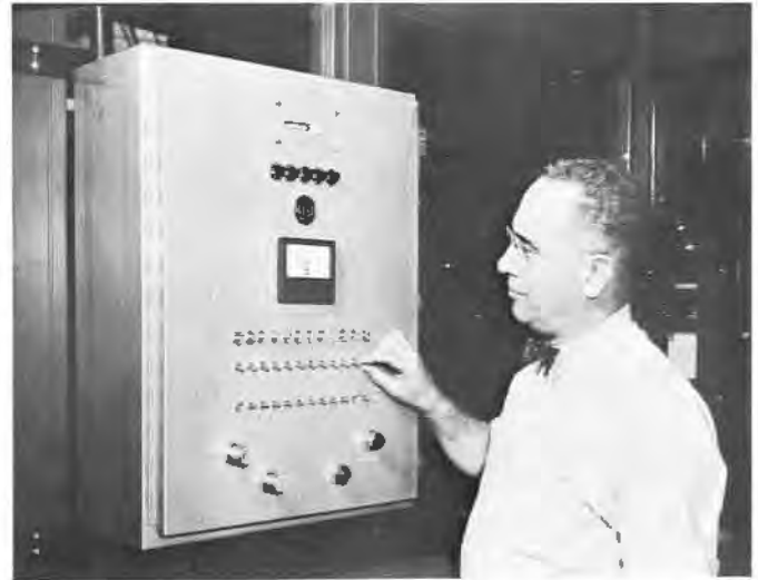
RCA Newspaper Counting Systems provide instantaneous counts of deliveries from high speed presses. It counts up to 120,000 units per minute.
