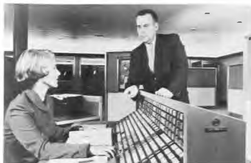
A supervisor instructs an operator at the RCA-501 control console.
