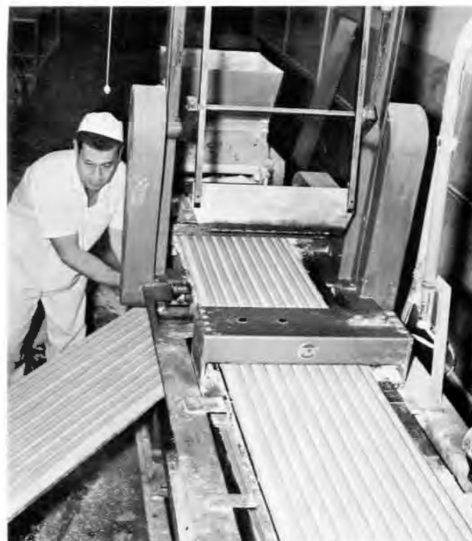
The RCA Metal Detector inspects sheets of powdered chewing gum at the Frank H. Flee Corporation.
