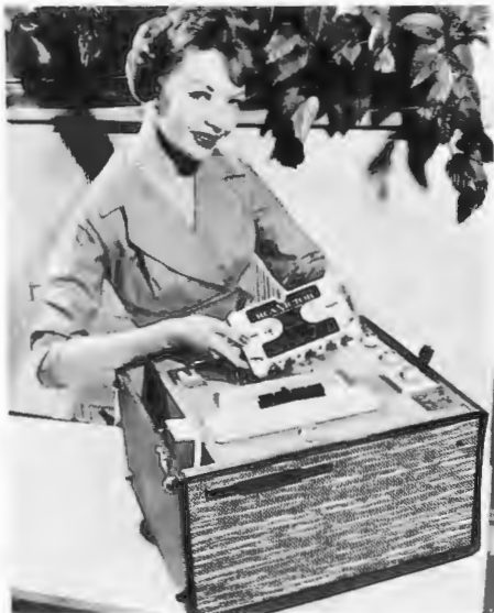
Semi-automatic stereo-tape player-recorder has easy-to-use cartridge containing one hour of stereo music or two hours of monaural.
