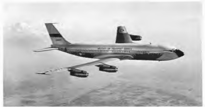
The VC-137A will operate above 40,000 feet; has a range of approximately 3,500 nautical miles.
