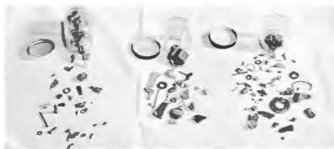
Typical metal particles in chocolate candy, spotted by an RCA Metal Detector, over an extended period of time.
