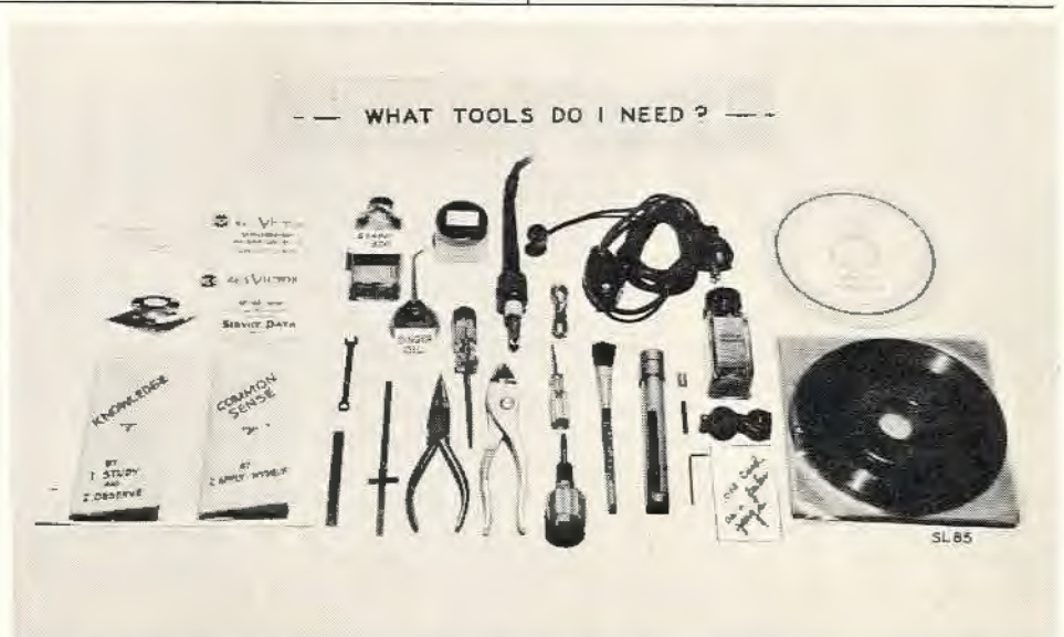
FIG. 1. A handful of major aids are required to service RCA's simplified record reproducing system.
