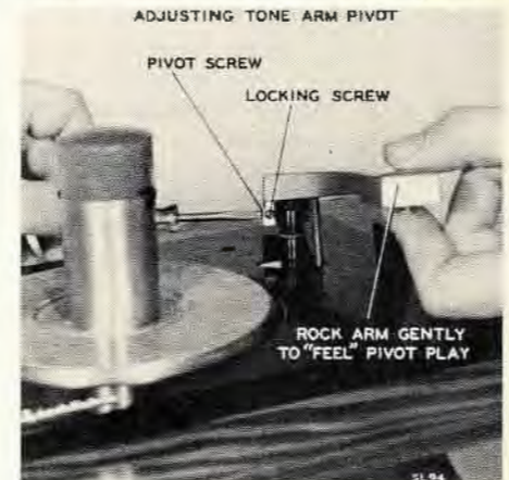
FIG. 4. Proper adjustment of tone arm pivot is important to change and play operations.
