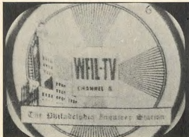
Fig. 3 The snowy appearance of this picture shows the result when the signal is extremely weak.
