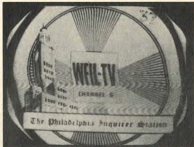
Fig. 4 Dialhermy interference produced the picture distortions shown above.
