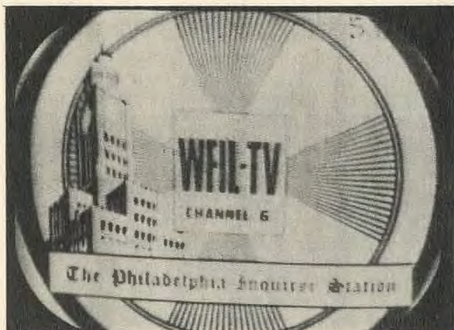
Fig. 2 The signal has been attenuated to a point where its weakness is becoming apparent.
