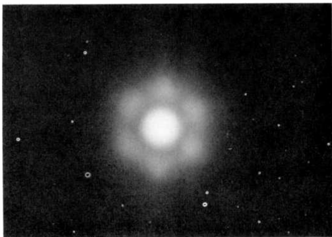
Fig. 4—Transmission-diffraction pattern of a latex plane-parallel cell using an He-Ne laser.
