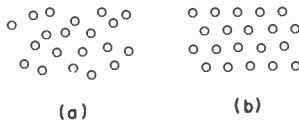
Fig. 1—Schematic views (a) of disordered and (b) of ordered states of latex dispersion.
