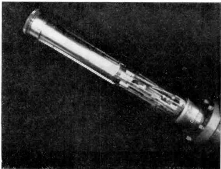
Fig. 10(a)—Photograph of experimental silicon cold-cathode vidicon tube.
