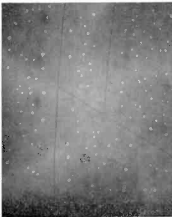
Fig. 3—Optical micrograph of a heat-treated thick \text{Al}_2\text{O}_3 film showing pinholes and line cracks (approx. 200 \times before reduction).
