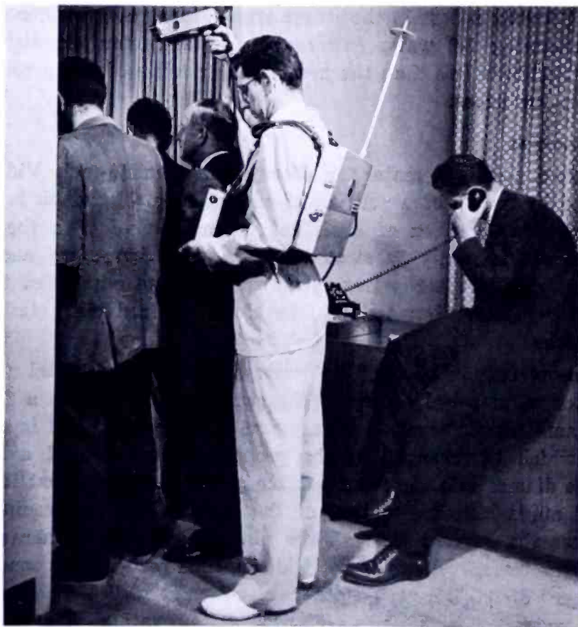
Fig. 7—Operation of the TCP with the monitor detached from the camera.
