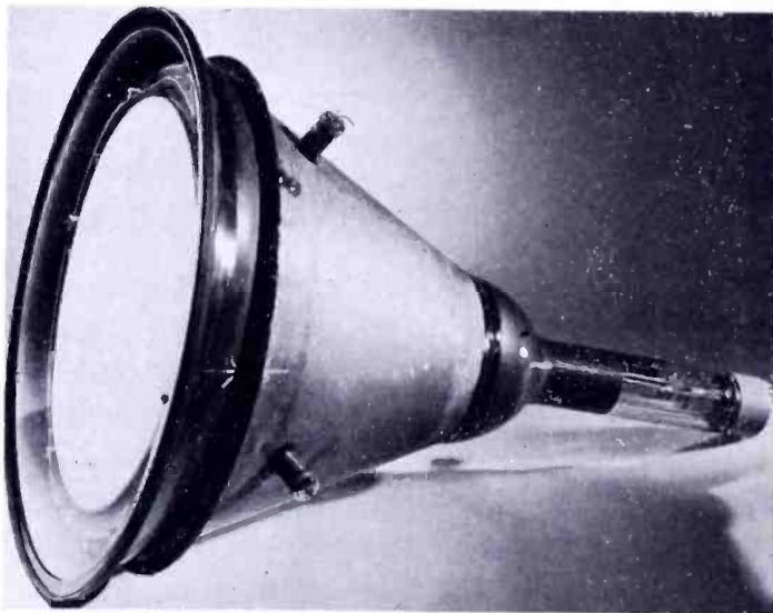
Fig. 1—Direct-view storage tube with 10-inch-diameter target.
