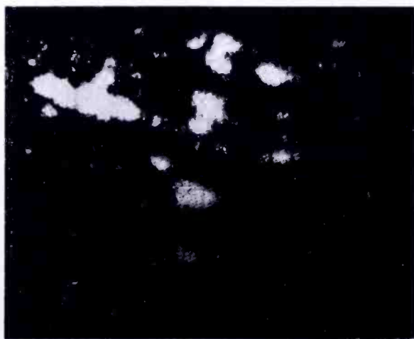
Fig. 9—Photograph of portion of projected radar display showing stored noise.
