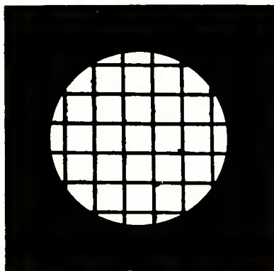
Fig. 1—Photomicrograph of 200 mesh per inch screen stretched across grid aperture.
