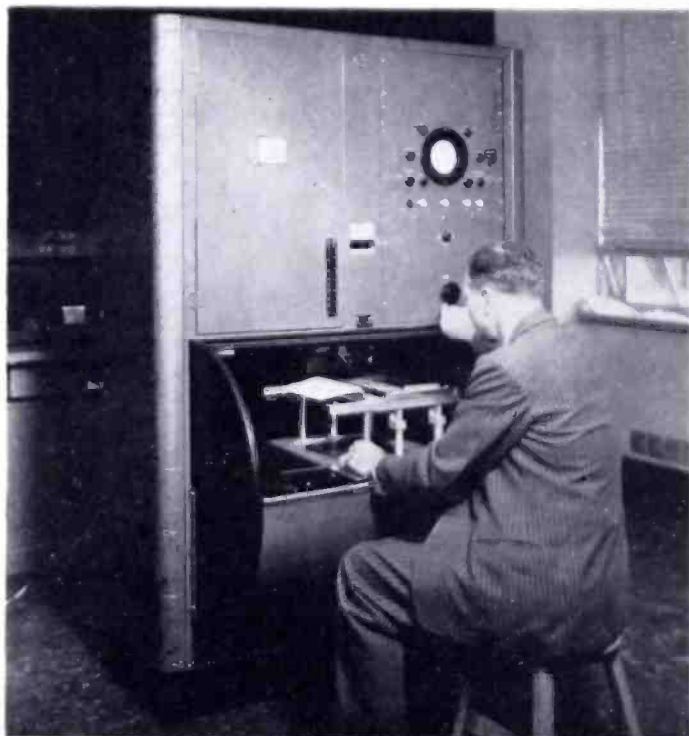
Fig. 2—Loading the flat-bed scanner.
