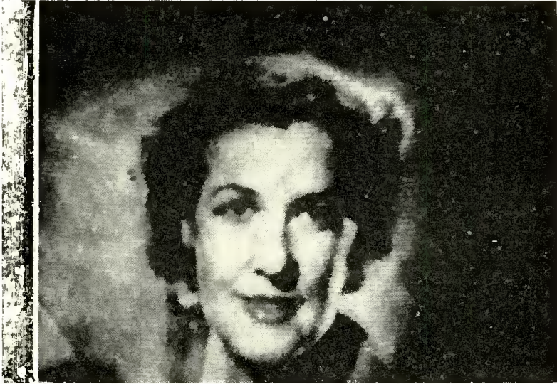
Fig. 9—Quality of a stored halftone picture. Viewing duration is from one to ten seconds, depending on the residual gas pressure.
