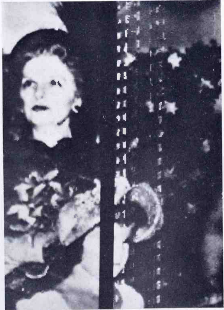
Fig. 6—Interference reduction obtained by reducing bandwidth. Left portion 1.3-kilocycle i-f bandwidth; right portion, showing diathermy interference, 4-kilocycle i-f bandwidth.
