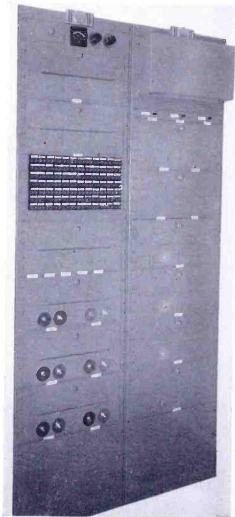
Fig. 2—Racks containing all necessary amplifiers, power supplies, and relays for the audio system.
