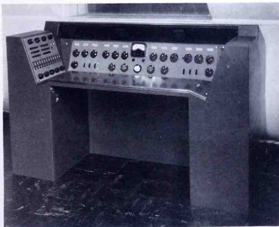
Fig. 1—The studio console shown in position with video monitor housing attached.
