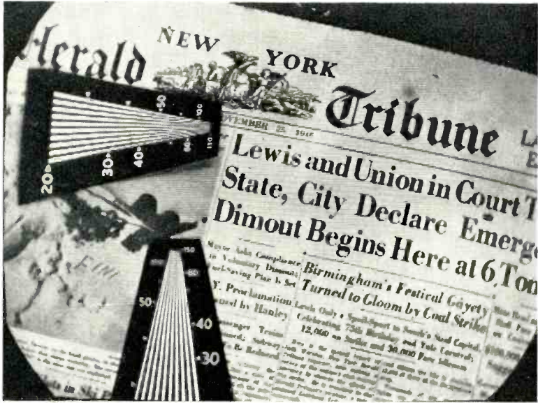
Fig. 34—400-line television picture with small scanning apertures in camera and kinescope.
