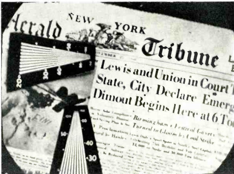
Fig. 35—400-line television picture with scanning apertures increased to give a "flat" field in camera and kinescope.
