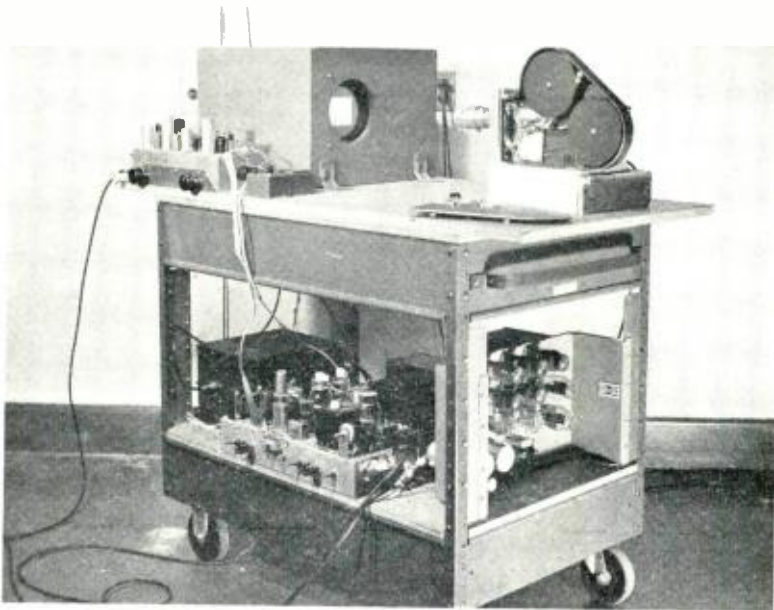
Fig. 2—"Breadboard" camera and photographic monitor.
