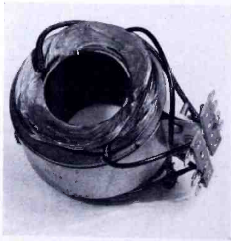
Fig. 17—First developmental sample deflection yoke with molded iron dust core in place.
