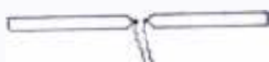
Fig. 9—Single composite dipole, driven and auxiliary elements considered to be connected in parallel.
