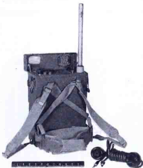
Fig. 3—Walkie-talkie transceiver (SCR-300-A).
