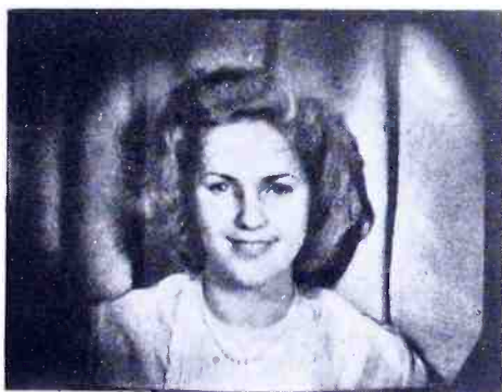
Fig. 11—Television Picture Taken with the Subject Illuminated by 3 Kilowatt Incandescent Light.
