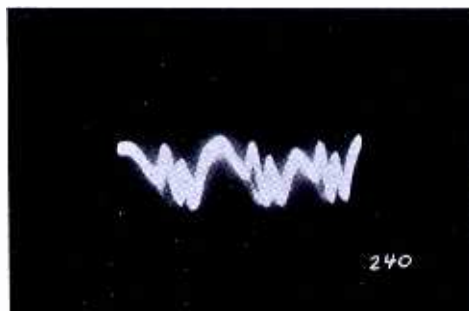
Fig. 25—900 cycle low pass filter output using one receiver with 2000 cycle intermediate frequency bandwidth. 180 cycle revs were used with 720 cycles shift.
