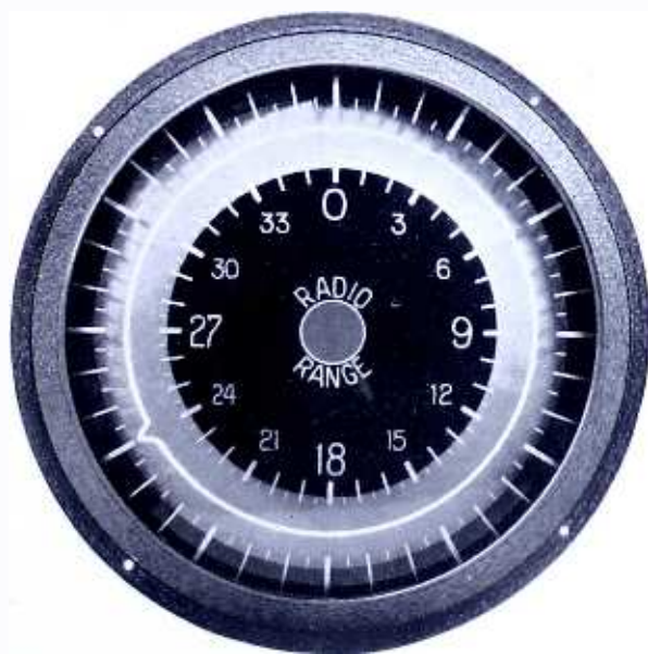
Fig. 5—Face of omnidirectional-range azimuth indicator. A bearing of 240 degrees is indicated.
