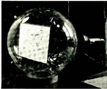
Fig. 2—12-inch direct-viewing television cathode-ray tube for large light output at high contrast.
