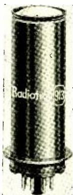
Fig. 2—The new midget, low-voltage, high-vacuum, cathode-ray tube.
