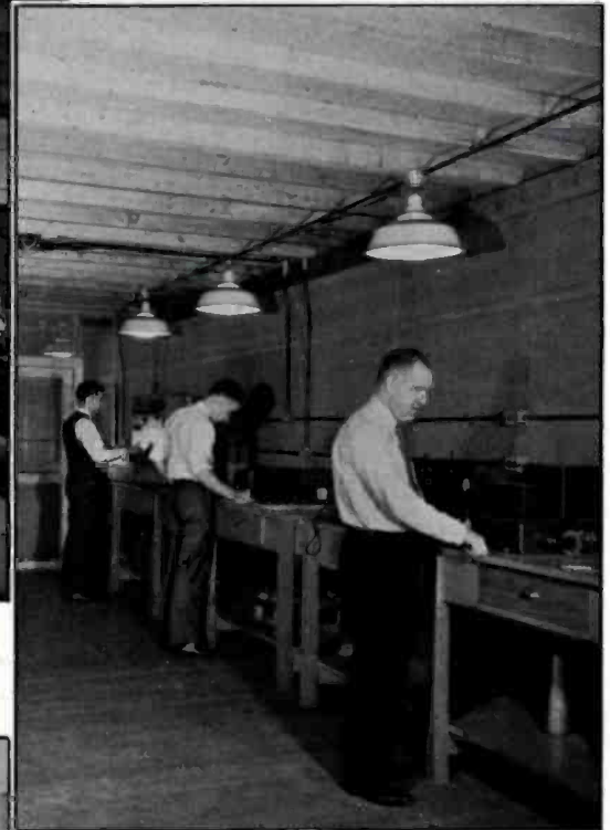
Shielded Test Room, for making sensitivity and selectivity radio-frequency tests
