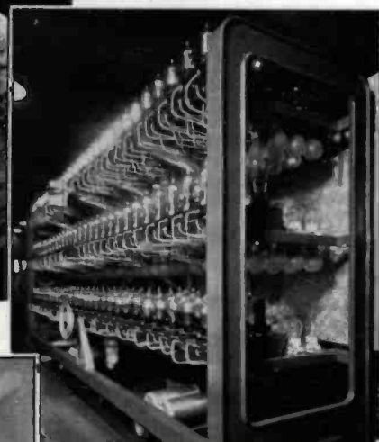
Seasoning and degassifying racks, where Radiotrons are "tempered" for stabilization of characteristics
