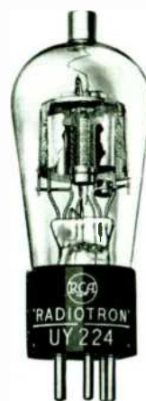
Fig. 5 Illustrating the position of the heater in the RCA Radiotron UY-224
