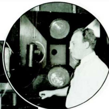
The television and transmitter pick-up arrangement used by the General Electric Company
