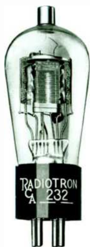
Fig. 3 The much used screen grid construction
