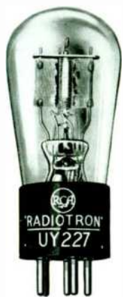
Fig. 4 Mount of RCA Radiotron UY-227 cut away to show position of heater
