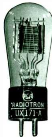
FIG. 2 Showing the elements of typical three- electrode tube
