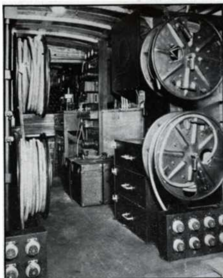
Interior of portable recording truck of RCA Photophone used on all RKO features made outside studios
