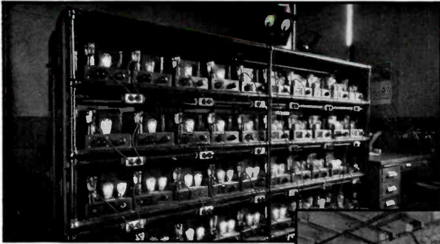
A check test on rectifier RCA Radiotrons. Rectifier RCA Radiotrons make possible A-C operation
