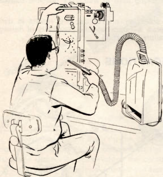
Figure 4—Remove Dirt and Dust from Chassis
