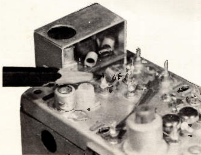
Figure 6—KRK 142 Tuner Showing MOS-FET
