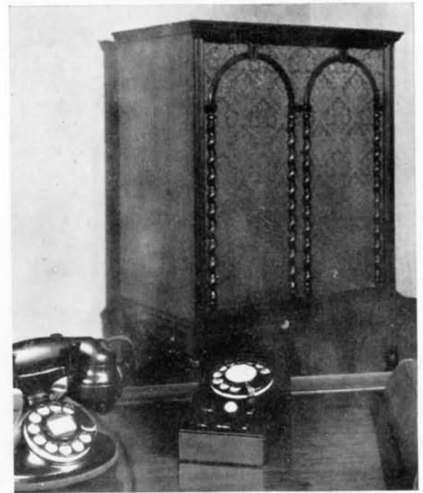
Figure 30. Typical office monitoring installation showing high fidelity loudspeaker and dial program selector which permit the executive to listen to any studio in the building and to any of the more important local stations.
