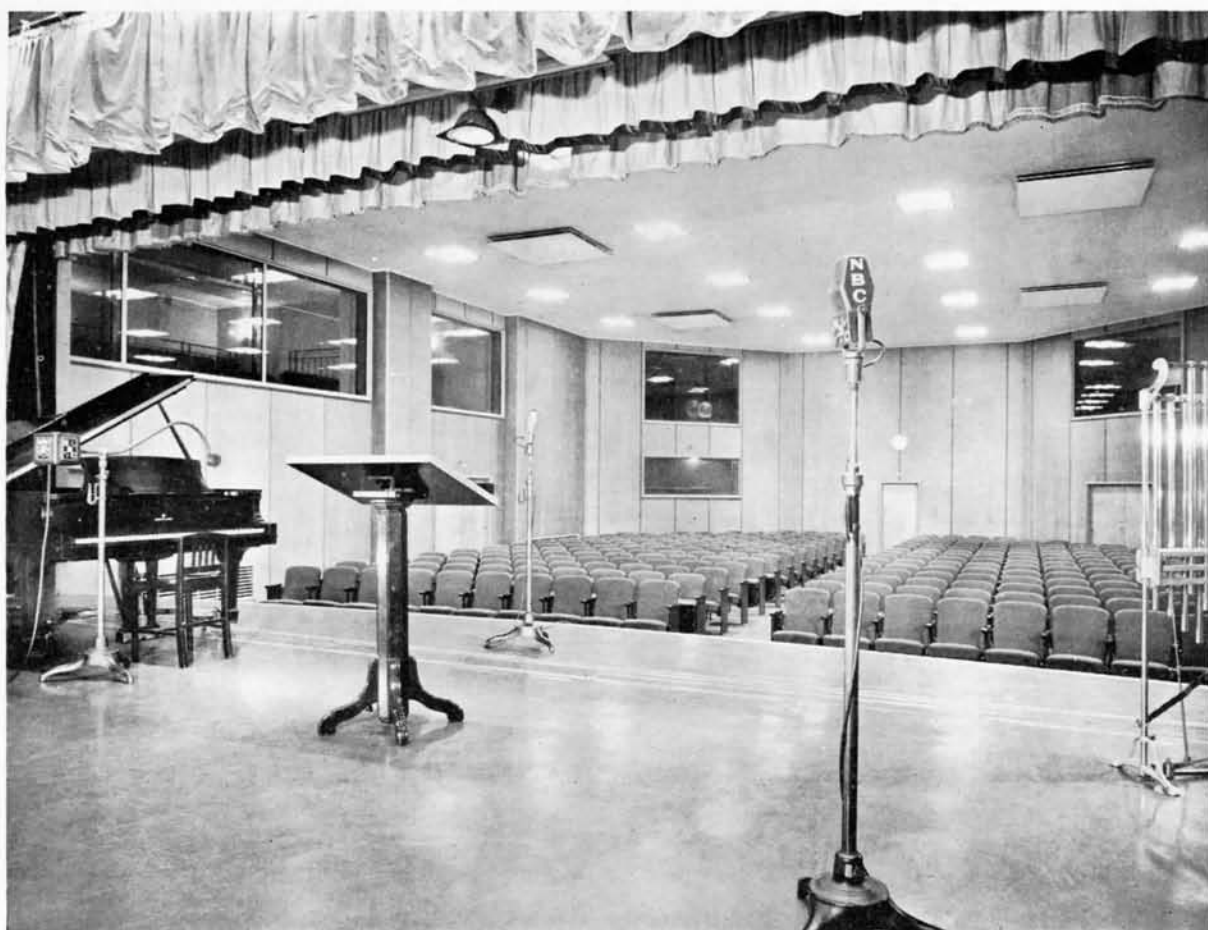
Figure 23. Studio 8G, 50' x 89' x 19', built like a miniature theatre. A glass curtain slides from the wings to isolate the stage from the audience.
