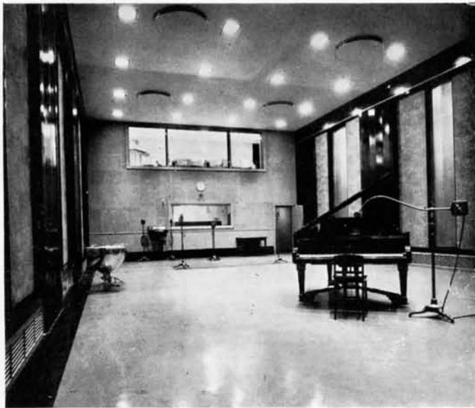
Figure 19. One of the 30' x 50' x 18' studios on the third floor, showing the sliding acoustical panels partially open.
