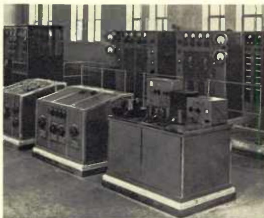
GENEVA —Program goes direct by wire from Salzburg to International Transmitter like this at "Radio Nations," Swiss Government transmitting station located at Geneva. Here it is put on what engineers call "short wave" to RCA Communications receiver in U. S.
