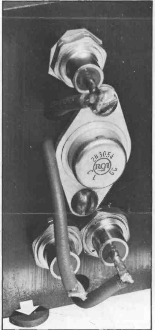
Figure 4: Closeup of left side of heat sink shows how it is insulated from the chassis by fiber shoulder washer (arrow). Note how hexagonal mica insulator is placed under diode, D_1 , shown at top. The same arrangement should be used in mounting diode, D_4 , on the right side of the heat sink.
