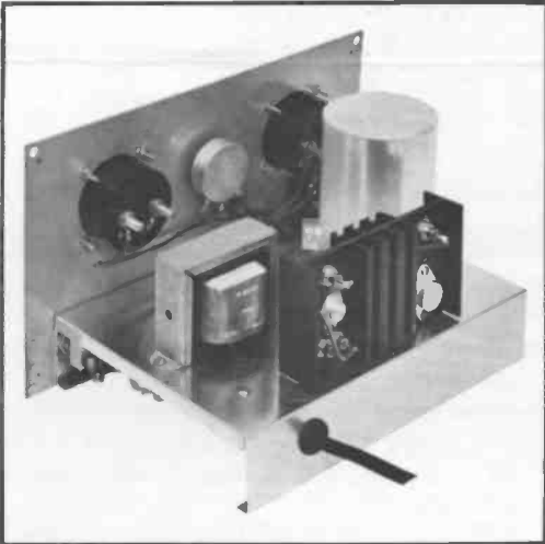
Figure 2: Rear view of W2OKO's power supply shows layout arrangement of four power diodes and 2N3054 and 2N3055 transistors on heat sink. Builders are advised to leave sufficient room around heat sink for air circulation.
