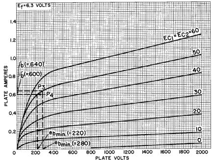
Figure 1: Typical plate characteristics of type 7094 triode connection (grid No. 1 connected to grid No. 2).
