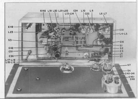
Fig. 2. Inside view of the transmitter. Note the area where the paint is removed from the panel for contact with the chassis. Also note the meter shield, the meter by-pass capacitors, and the shielded power leads—all essential TVI precautions.
