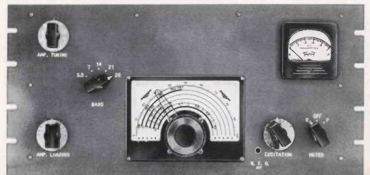
plifier. A keyed amplifier between the VFO and the first frequency multiplier eliminates any back-wave and permits full break-in operation.
