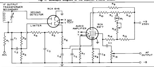
Fig. 1. Schematic diagram of the superhet S-meter circuit.
