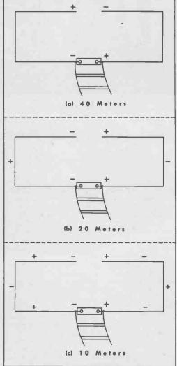
Fig. 2. Maximum voltage points on the ontenno for 40-, 20-, and 10-meter operation.
