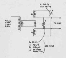
Fig. 3. Circuit of the ontenna coupler used with the all-band antenna.
