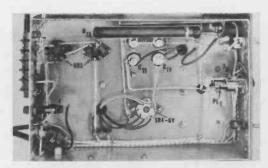
fig. 4. An example of neat wiring. Note that  $R_{13}$  is mounted above  $R_{12}$  to permit easy access to the adjustoble slider.
