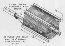
Fig. 3. Recommended method of connecting the coaxlal transmission line to the antenna link. The additional Lucite strips keep the link from touching the tank coil.
