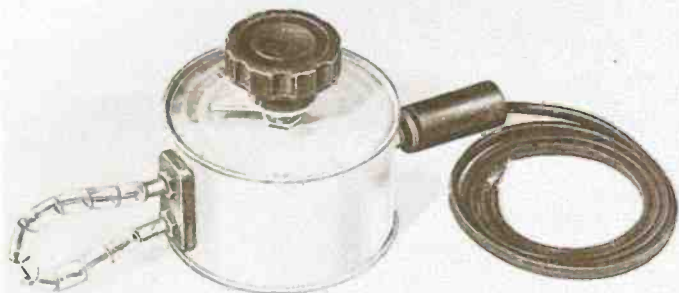
Despite its humble origin, this easily built but extremely sensitive absorption type wavemeter is a "must" for tracking down offending harmonic radiation in transmitters.
