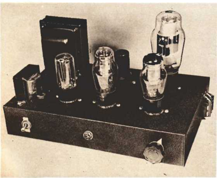
The electronic bias supply shown above provides a regulated bias voltage adjustable from 30 to 80 volts and handles a rectified grid current up to 200 ma.
