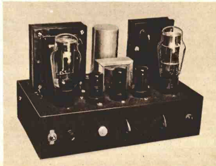
This functional looking speech amplifier delivers 12 watts of actual power output to a load at less than 4% distortion.
