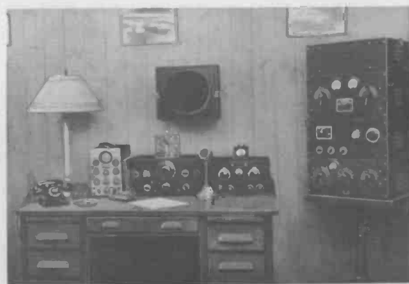
W3NT of Norfolk, Virginia, wins the five-spot for one of the neatest layouts we have seen in a long time. The business end of the station consists of two separate exciters. The final uses a pair of RCA-860 screen-grid types. Each exciter may also be used separately as a portable rig. Total tubes in transmitter amount to nearly thirty . . . and they are all RCA!
