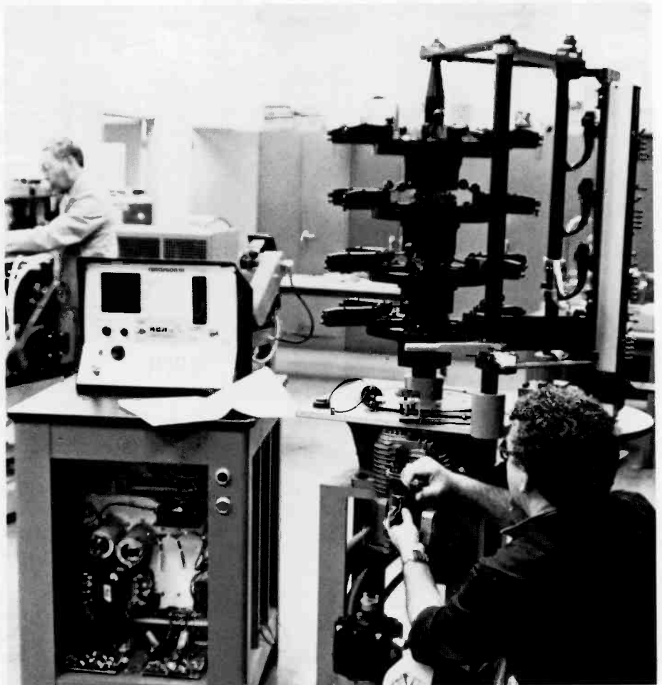
Fig. 10. Four-level production winder for toroidal-type vertical deflection coils under construction in the Equipment Development machine assembly lab.
