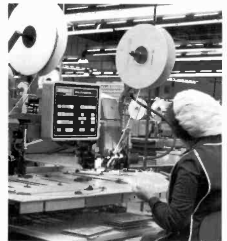
Fig. 2. The VCD machine inserts parts from sequenced reels into each circuit board.
