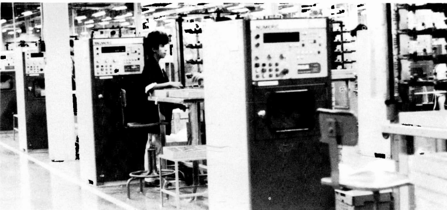
Fig. 20. Machines designed for the Torreon production facility: (a) high-voltage transformer primary coil stick winders; (b) saddle coil winding machines; (c) toroidal coil winding machines.
