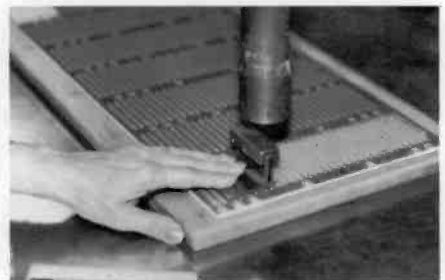
Fig. 2. Compliant pins are inserted into PC boards using presses of this type. A vibrating conveyor shakes pins into the connector shell holes, and the press attaches the pins housed in the connector shell to the board as a unit.
