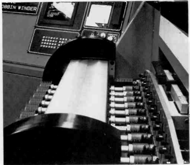
ROSE production winder for tertiary coils. Winding on the right, load and unload on the left.
