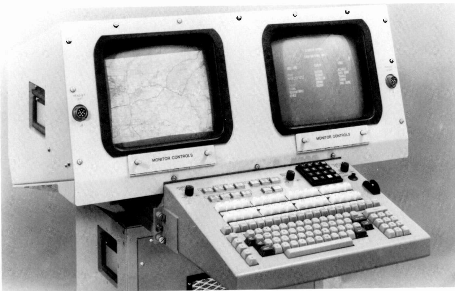
Fig. 1. RCA military colorgraphics workstation. This is an upgraded version of an AN/TSQ-130(V), showing alphanumeric database information on the right screen and electronically-stored maps with colorgraphic overlay displayed on the left screen.
