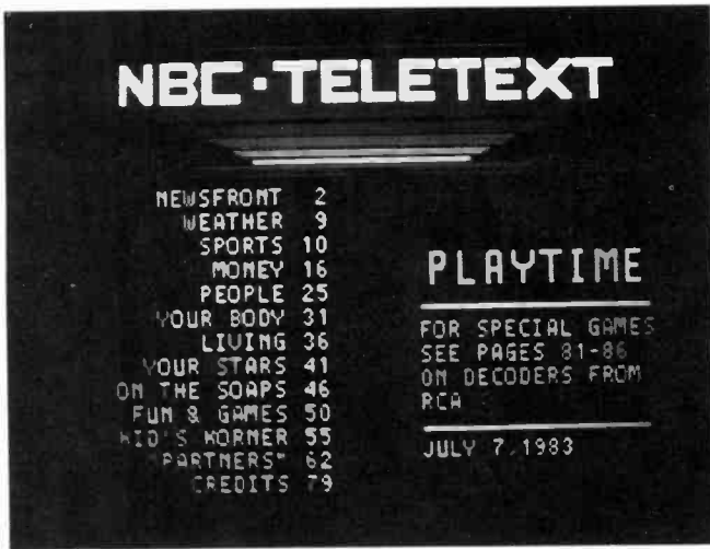
Fig. 1a. The main NBC index page. The primary character set was used to produce the small text and numbers. The larger "PLAYTIME" was constructed using the double-size control from the C0 control set. The different font in "NBC TELETEXT" was constructed using lines with a larger logical pel. The colored shapes underneath the title were constructed using filled polygons (see color versions on back cover). The text of the contents is presented on a light gray rectangle drawn with highlight turned on to produce the blue border. Additional blue lines were drawn to give the appearance of overlapping rectangles.
