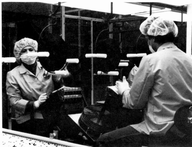
Fig. 3. Conveyor loading. The surface-treatment-line conveyor is loaded with VideoDiscs.
