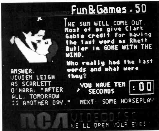
Fig. 1c. A page from the fun-and-games section. A series of one-second wait standards were used to produce a clock counting down from 10 to 0, at which point the answer was automatically shown.
