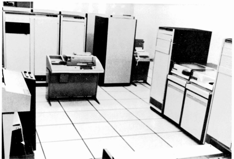
Fig. 5. ATSJEA computer room and test stands, comprising a system for testing jet engine fuel controls.
