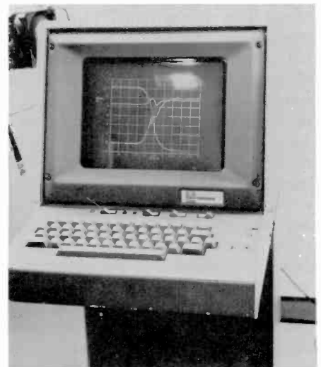
Fig. 4. CRT graphics terminal displaying averaged color transition waveforms.
