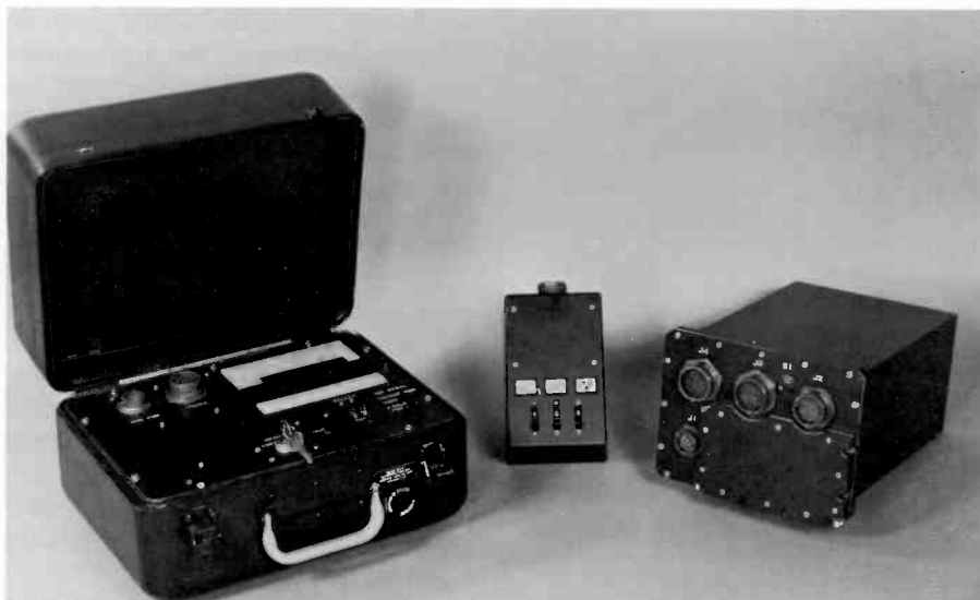
Fig. 8. Vehicle Monitoring System hardware, boasting 32,000-word memory, aids study of vehicle use, abuse, and maintenance.
