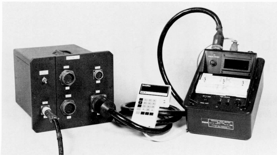
Fig. 14. Simplified Test Equipment for the Army's XM1 tank contains 190,000 bytes of memory and has expansion capability.
