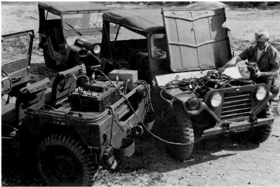
Fig. 6. Automatic Test Equipment/Internal Combustion Engines, shown in operation on Army vehicles.
