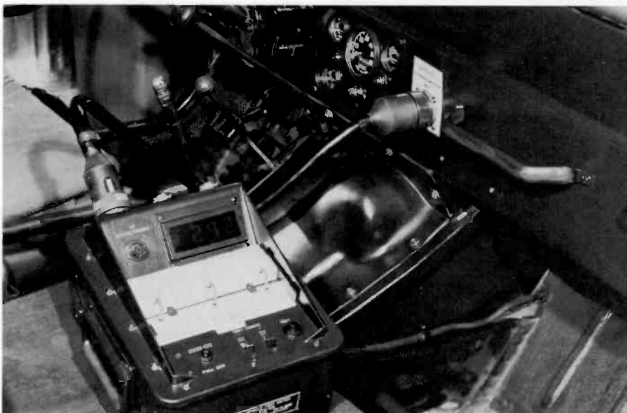
Fig. 9. Simplified Test Equipment (STE/ICE) is small and easy to use, yet performs hundreds of mechanical and electrical tests.
