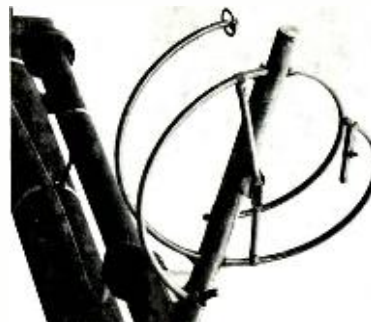
Fig. 5—Two resonant half-wave dipoles are curved into one-turn helices and interlaced to maintain constant current for omnidirectional service.
