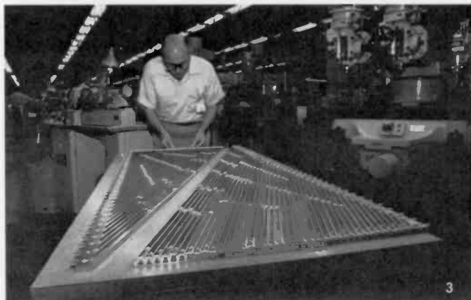
Fig. 2 shows the two identical housings for right and left distribution networks, fabricated as part of an IR&D effort. The NC-milled grooves forming the outer conductors for the coaxial lines are visible on the right. Installation of tubular center conductors supported by Teflon beads is shown in Fig. 3.
