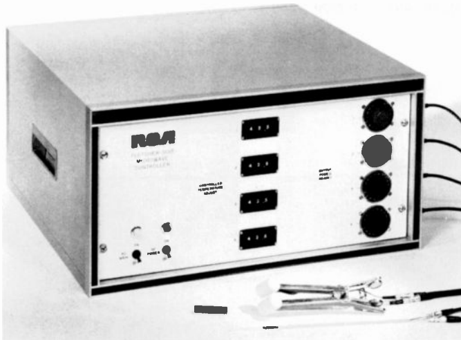
Fig. 4. The modified Fletcher-Suit system for treating cancer of the cervix and uterus with ionizing radiation and microwave hyperthermia. The system includes a 50-watt magnetron source, a four-way power-splitter/controller, and output attenuators.
