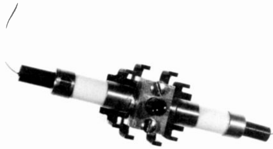
Fig. 2. A 10,000-volt package with 10 diodes in series.
