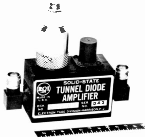
The RCA tunnel-diode amplifier is an example of fast-turnaround engineering. Tunnel diodes were still in the relatively early stages of development when the amplifier was developed and introduced into commercial production for communications and radar systems. The amplifiers used diodes developed and manufactured at the RCA Somerville, N.J., plant. The model shown was used as a retrofit in the C-band RCA weather radar, and served to increase the operating range of the system by substantially decreasing the receiver's noise figure.
