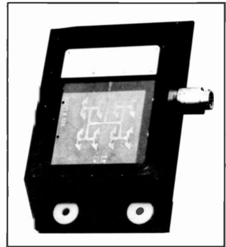
Fig. 7. The cast-aluminum radar-speed-sensor housing with the protective faceplate removed shows the printed circuit dipole array antenna and the coverplate that shields the microwave oscillator and mixer.
