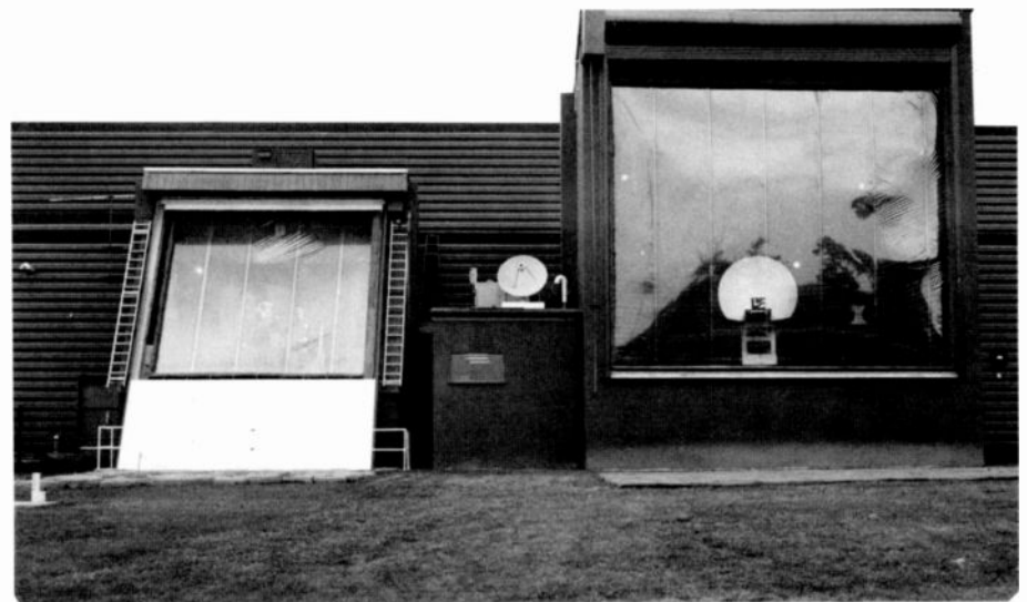
Fig. 11. An internal view of the RCA Astro-Electronics 400-foot range, dual anechoic chambers, showing the Satcom E spacecraft (on the left) and the developmental model Satcom F antenna (on the right) undergoing rf testing. The room, located between the chambers, houses the automatic antenna analyzer and other ancillary test equipment.
