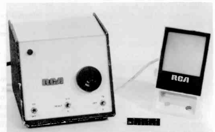
Fig. 10. A Doppler radar used as a noncontacting apnea monitor. The unit on the right contains the antenna, transmitter, receiver, and signal processor; the unit on the left contains an audible alarm that can be activated when and if respiration ceases. The unit operates at a frequency of 10.525 GHz.
