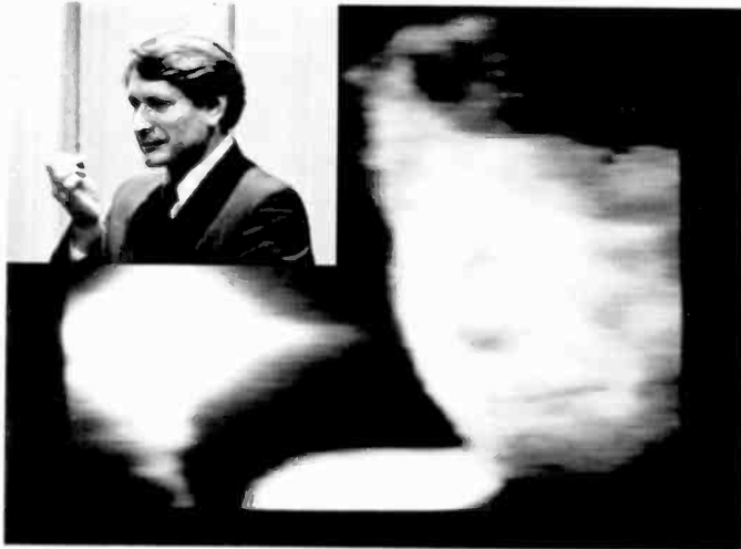
Fig. 12. Demonstration of the control of blooming in a Schottky-barrier IR-CCD image sensor. Thermal image of Walter Kosonocky holding a glowing match detected by a 64-by 128-element PtSi IR-CCD TV camera (right). Visible photograph of the scene (left).
