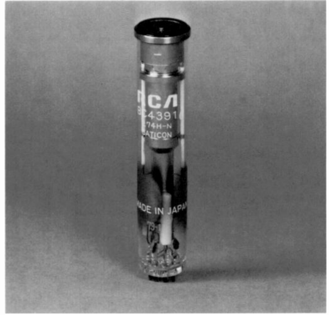
Fig. 4. The new low capacitance Saticon tube (BC4391) showing the low-output-capacitance target contact.
