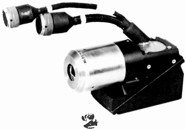
Fig. 1. This high-performance miniaturized TV sensor was developed for use on the Target Acquisition and Designator System/Pilot's Night Vision System (TADS/PNVS). Extensive use of hybrid circuitry resulted in this compact design (less than 1.0 kg).
