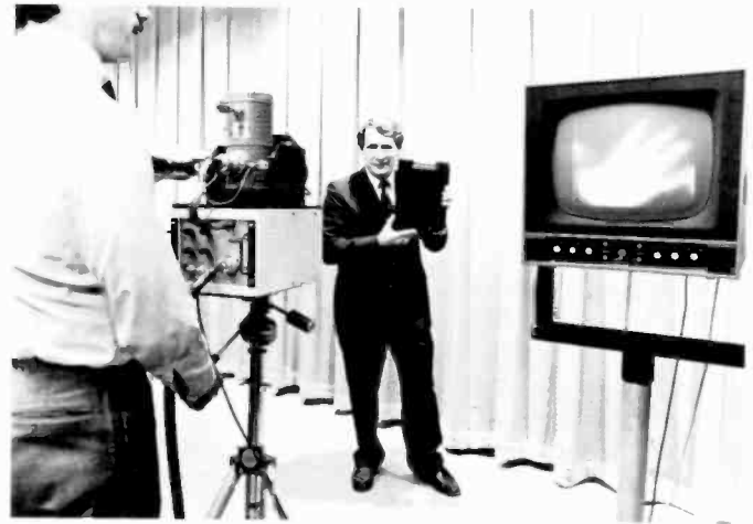
Fig. 13. Demonstration of the sensitivity of the 64 by 128 PtSi IR-CCD image sensor. In this experiment Walter Kosonocky is holding in front of the IR-CCD camera a notebook on which he previously formed a print of his hand. The thermal image of the handprint is shown on the TV monitor. The IR camera is operated by Harry Erhardt.
