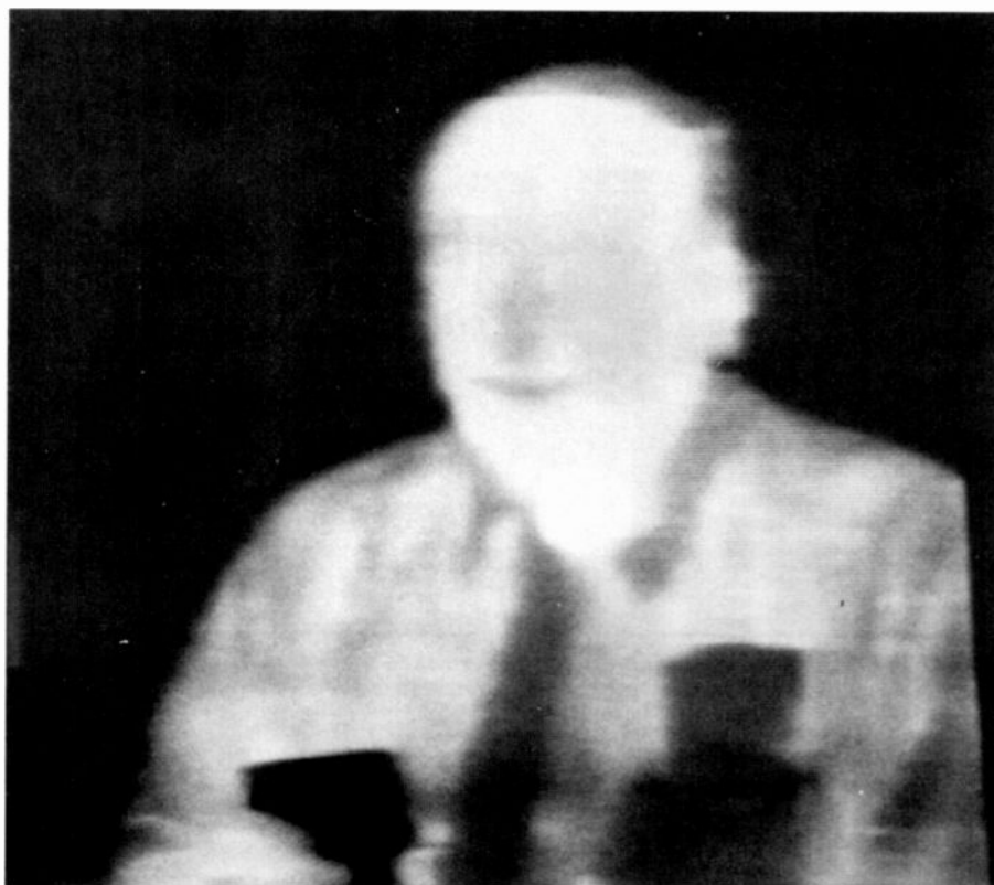
Fig. 5. High quality IR imagery obtained from a 64- by 128-Schottky-barrier FPA. IR imagery of high sensitivity and wide dynamic range has been obtained from 64 \times 128 Schottky-barrier FPAs.
