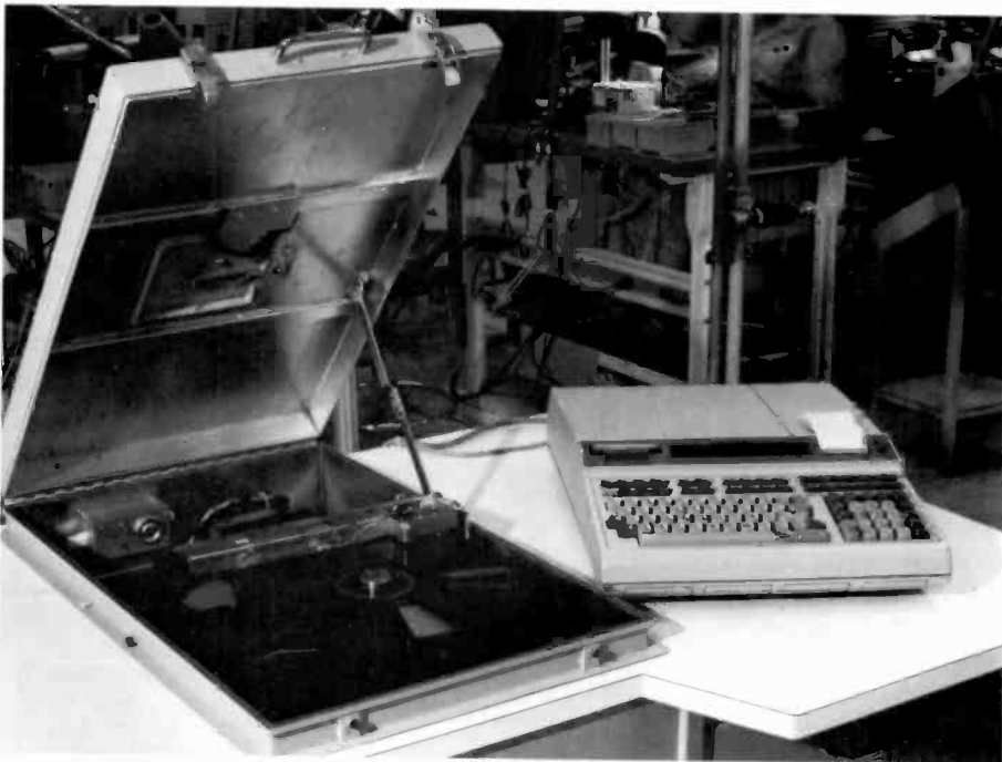
Fig. 4. The RFI enclosure's lid, shown in the disc-changing position, does not block access to the calculator, nor to the equipment bay.
