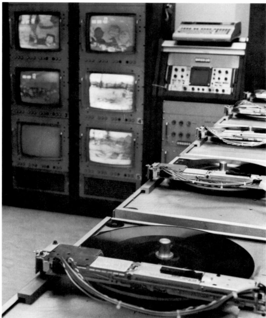
Fig. 1. A typical PET system showing television monitors, calculator, video signal-to-noise rack, and PET positions.
