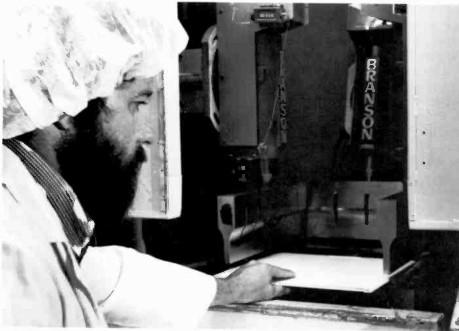
The ultrasonic welder machine. Three full-length horns are lowered simultaneously in a plunge-weld fashion.
