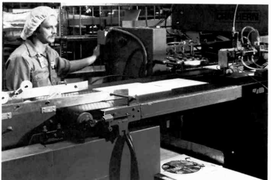
The label machine. The printed labels are applied, automatically, with a wet-glue process.
