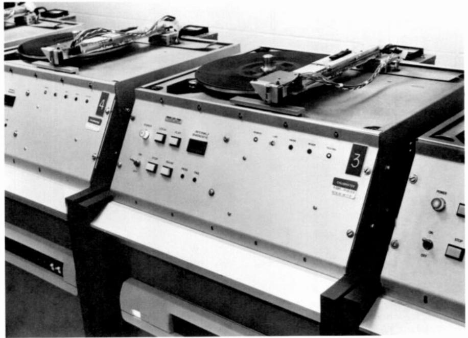
Fig. 2. A PET position showing precision turntable, front panel, and arm assembly.
