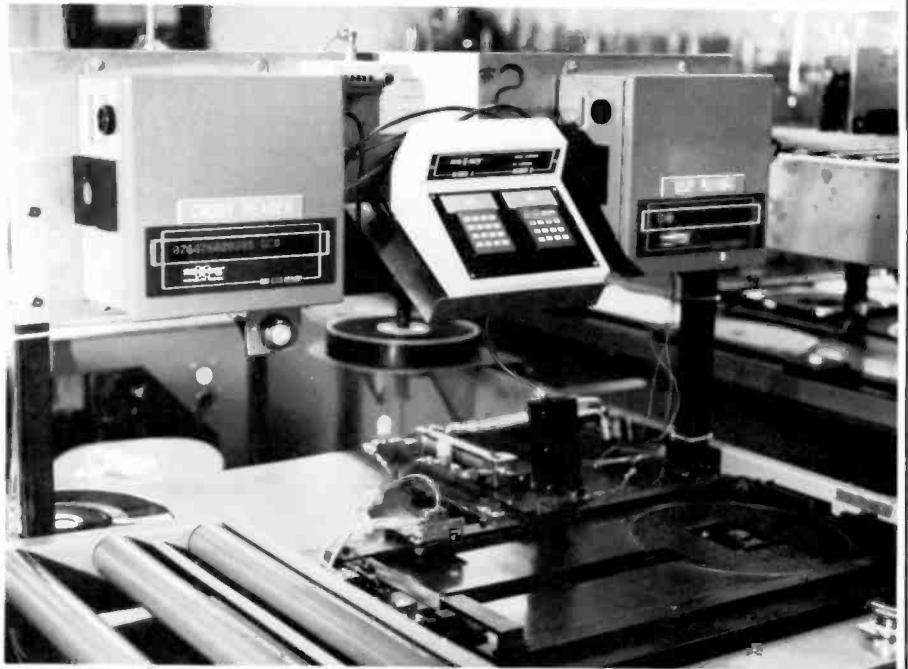
Bar code verifier system. This system electronically scans the bar codes on the caddy label and the disc, allowing automatic loading of the disc into the caddy when similar readings are registered on the displays.
