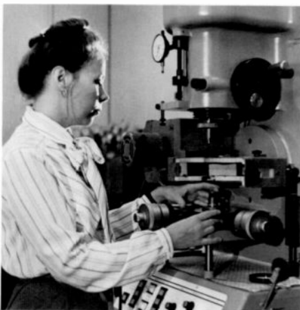
Fig. 4. The Rheometrics mechanical spectrometer is a versatile device that can subject the test sample to a variety of static and time-varying stresses at different temperatures, while monitoring mechanical response. Dynamic viscosity and elastic modulus are two parameters that can be measured.
