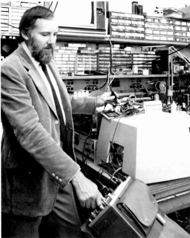
Author Ny debugging a microcomputer-based system in a "bare-bones" environment. Scope is in the foreground.
