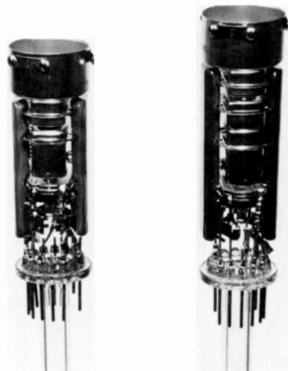
Fig. 11. Comparison of HiPI and bipotential gun size.
