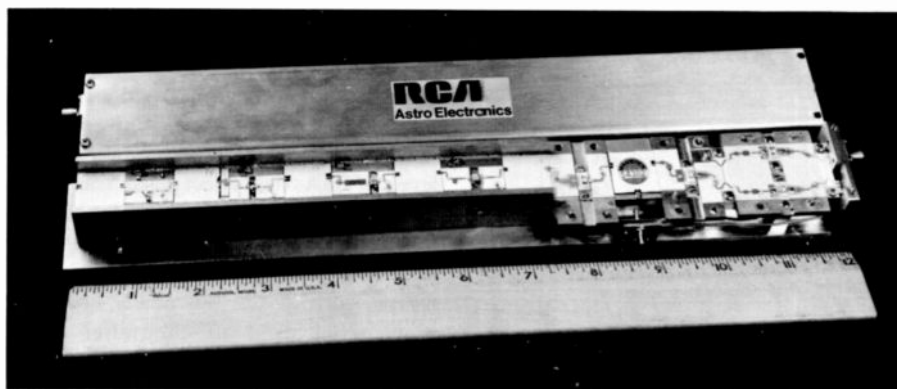
Fig. 6. The 5-W solid-state power amplifier laboratory model was designed and built to prove that GaAs FETs could replace TWTA's in spaceborne transponders.
