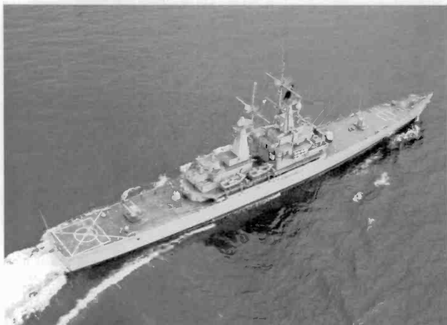
Fig. 5. USS Mississippi (CGN-40) underway. Radome of Gun Fire Control System Mk 86 Surface Search Radar, AN/SPQ-9, can be seen forward topside, Mk 45 gun mounts forward and aft, and dual-rail guided missile launchers forward and aft.
