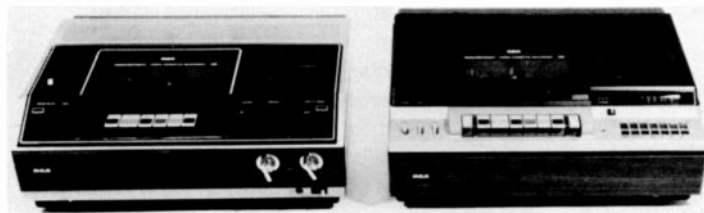
Fig. 2 The VK125 and VK250 cassettes are paperback book size, contain 125 and 250 meters of tape, and provide two and four hours of playing time respectively when used with any SelectaVision VCR.
