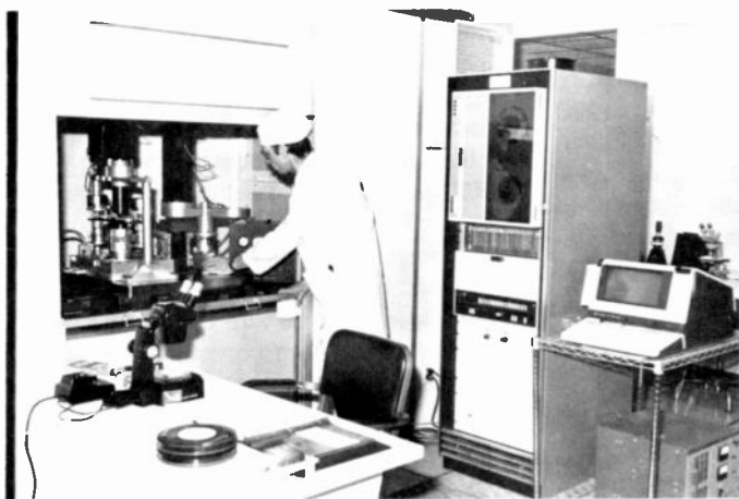
Fig. 10 The Electromask 2500, combination pattern generator and image repeater, makes possible the generation of a chrome reticle directly on the pattern generator and eliminates the contact-printing step previously required.
