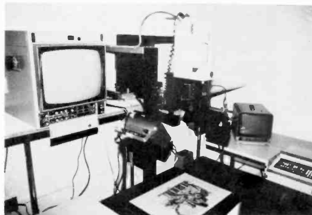
Fig. 2 Unique news show production system. RCA TK76 portable camera (top center); remote control panel (right); graphics stand (bottom).
