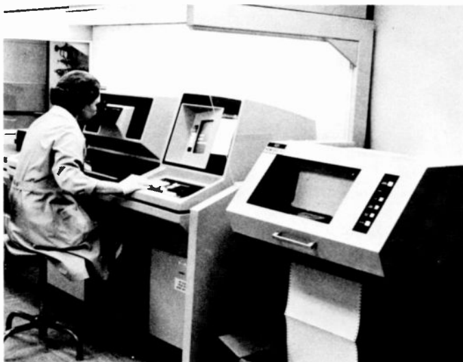
Fig. 8 The accuracy of defect-inspection procedures has increased through the use of equipment like this KLA automatic mask-inspection system.
