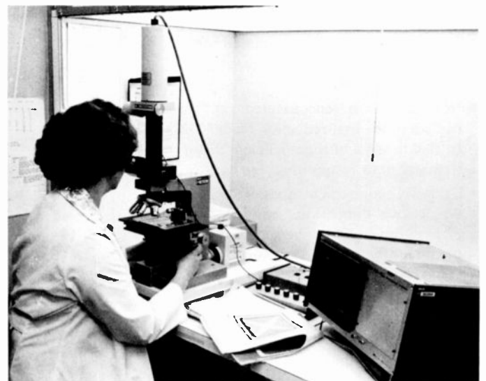
Fig. 9 This ITP electronic measurement system provides significantly improved accuracy in the measurement of mask-pattern elements.
