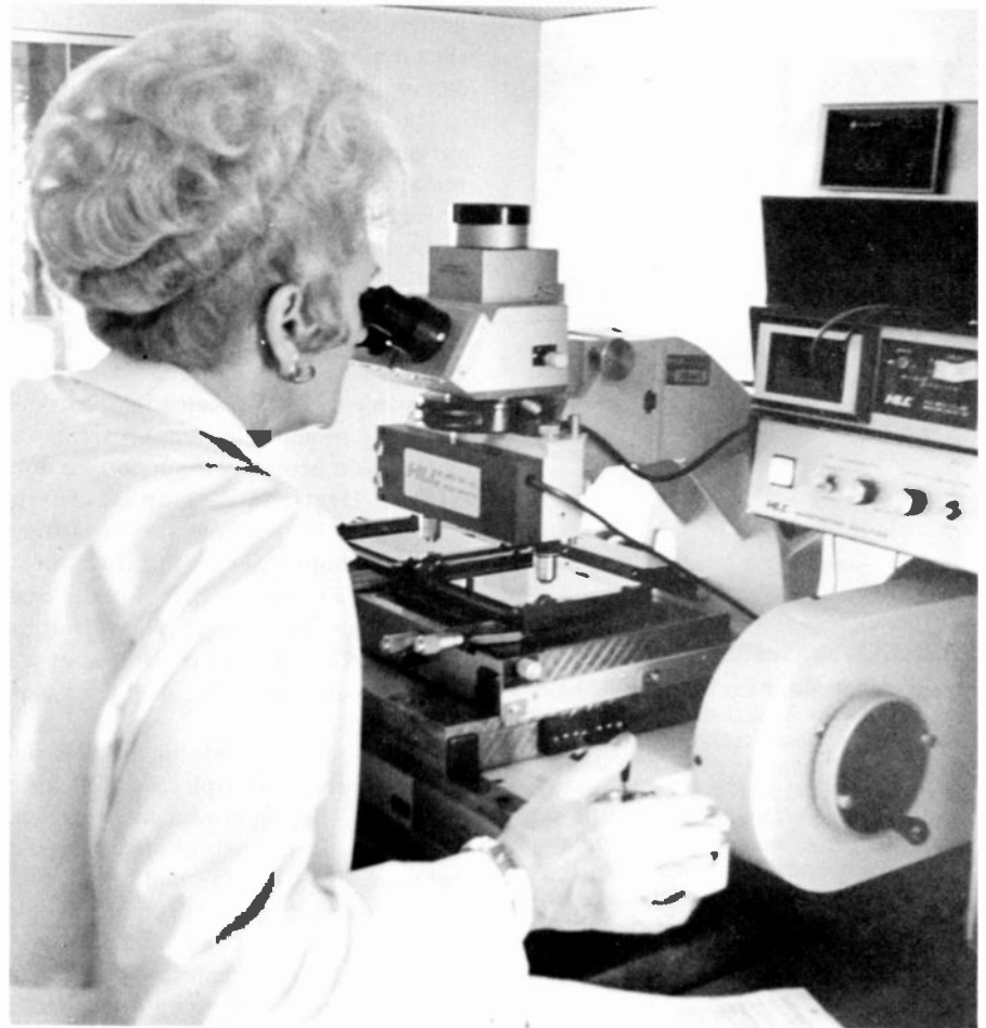
Fig. 4 The latest versions of equipment, such as this registration analyzer, assure precision of registration down to approximately 0.125 microns.
