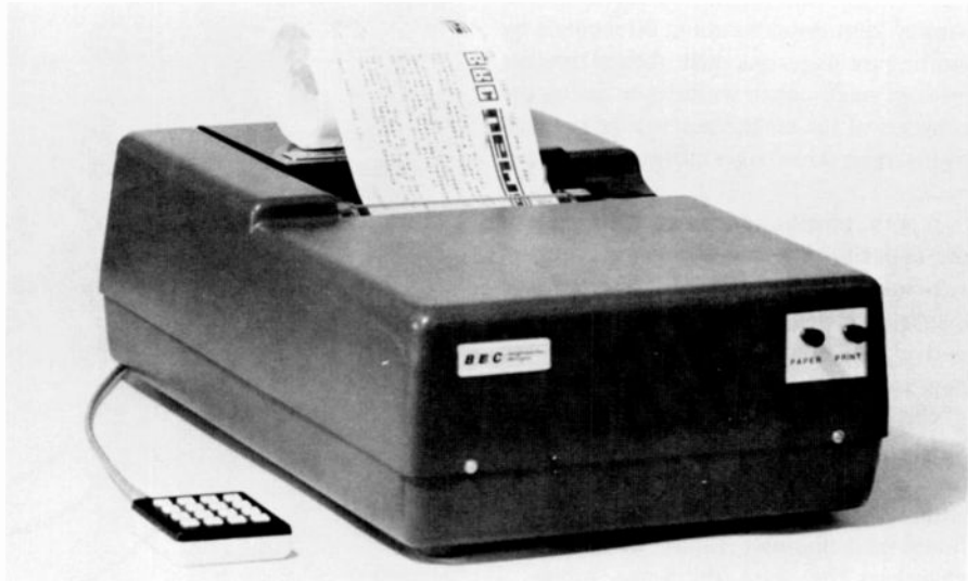
Fig. 6 Impact printer under development by BBC, prints any text or graphics page on paper within 35 seconds.
