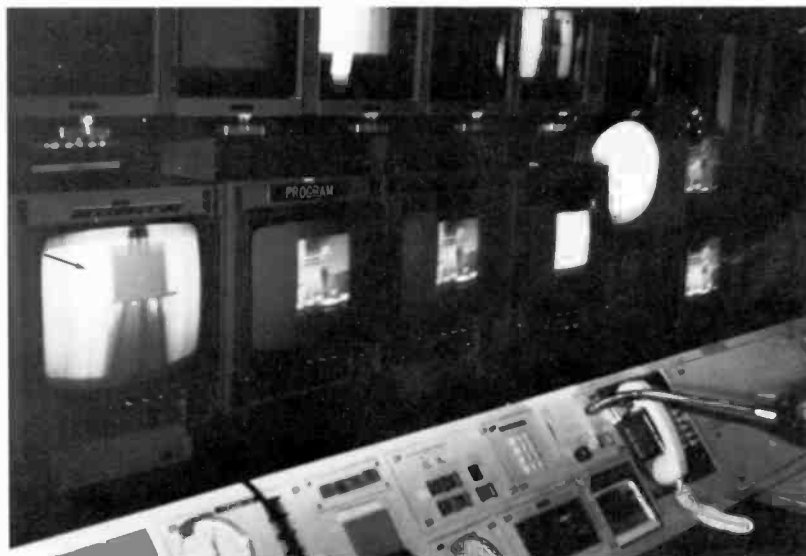
Fig. 11 Compressed picture derived from blue card on tripod (left-hand control room monitor).
