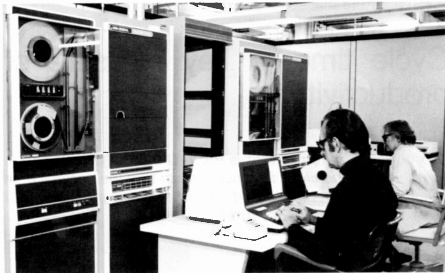
Fig. 3 The PMC computer room contains the minicomputer used to control the system.
