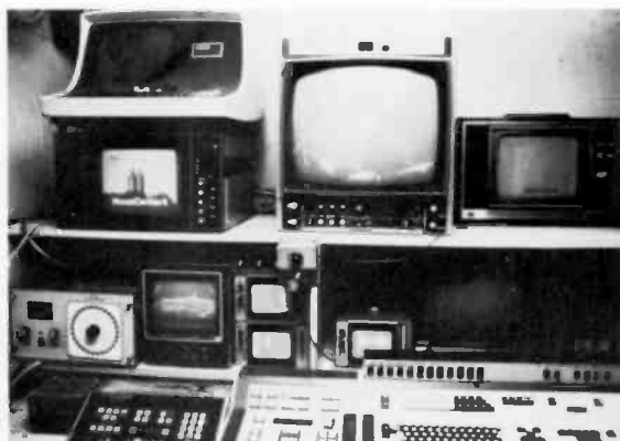
Fig. 5 Character generator room of News Center 4. Character generator keyboard is seen at bottom right; auxiliary control panel (bottom center); still store control panel (bottom left); ADDA terminal interface (top left).
