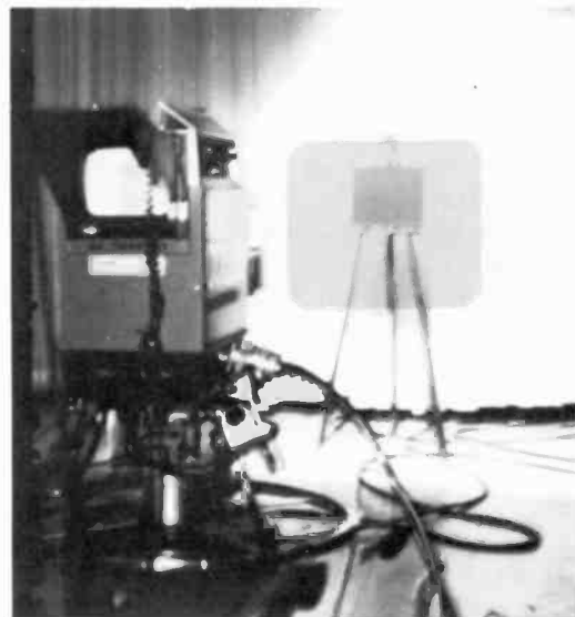
Fig. 12 RCA camera in studio and blue card on tripod for "chroma key".
