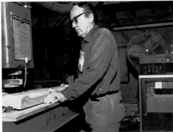
Fig. 4 Detail parts often have unusual shapes. This numerically controlled router can be reprogrammed for different shapes by changing the tape on the controller at the right. A typical tv cabinet has about 24 exposed detail parts; moulders, autoshapers, and tenon machines are also involved in this work.
