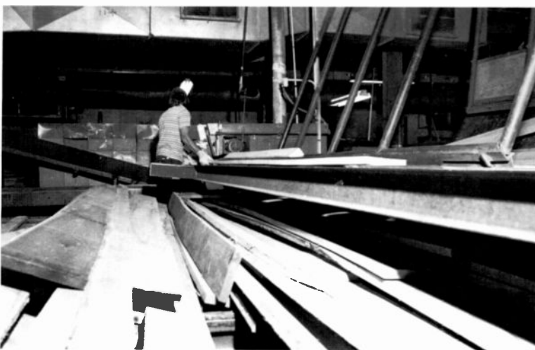
Fig. 2 Cutting to length is the first operation. The operator slides the lumber to the saw (at rear), picking out the best lengths and avoiding knots and bad spots in the rough lumber.
