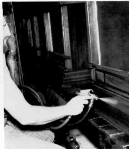
Fig. 10 Finishing requires many coats —three color coats and four sealing and top coats. The shading coat being applied here is combined with light detail sanding to provide a uniform appearance.
