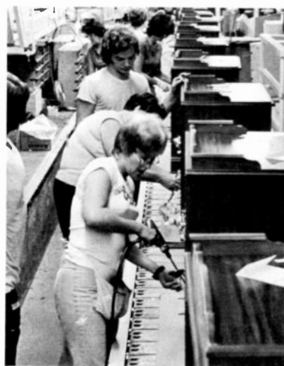
Fig. 9 (top left) Chassis being taken from the overhead monorail at left and being prepared for assembly to cabinets at right.
