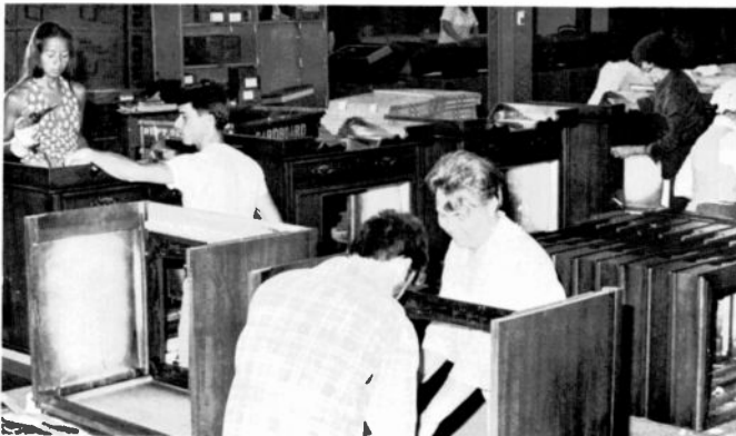
Fig. 3 Typical Cabinet Section assembly line. Knockdown cabinets are being assembled here.
