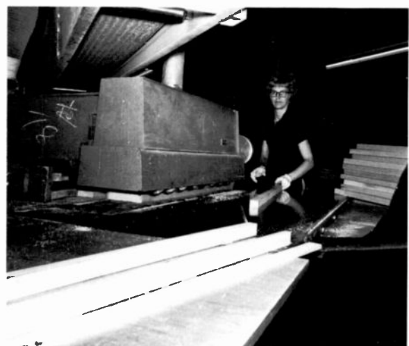
Fig. 3 Ripping is a two-person, back-and-forth operation. The operator sends the board through the saw to another operator (out of picture) who passes the cut portion back for another cut. A few seconds ago, this board was about 12" wide; now it's about six pieces like the one you see here.
