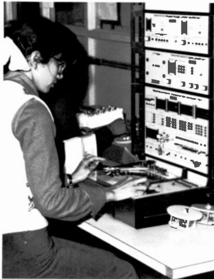
Fig. 2 Incoming material is inspected automatically whenever possible. Instrument shown is a transistor tester.
