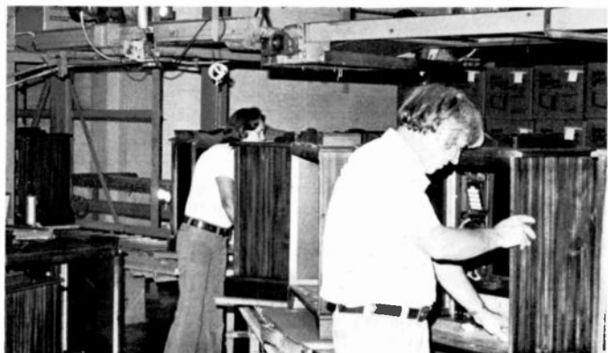
Fig. 4 End of the cabinet assembly line. The automatic elevator at the left takes the cabinets and cartons (on separate levels) up to the main floor for the rest of the assembly operations.
