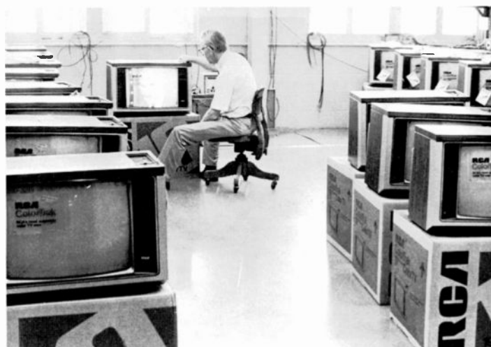
Fig. 16 (bottom right) Consumer Acceptance Analyst making the initial quality check on randomly selected 19-inch sets.
