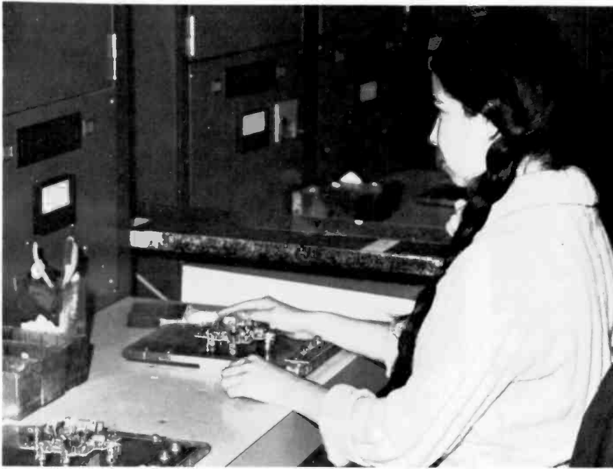
Fig. 7 Automatic test equipment checks out finished circuit boards very rapidly. Testers can test two boards independently. Display at top of cabinet gives commands to operators.
