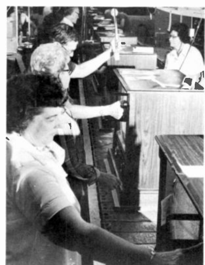
Fig. 9 (top left) Chassis being taken from the overhead monorail at left and being prepared for assembly to cabinets at right.
