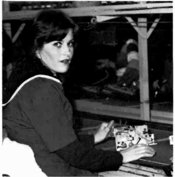
Fig. 10 Signal modules are assembled on a belt conveyor. Their metal frames hold seven smaller modules, an interconnect board, and wiring.
