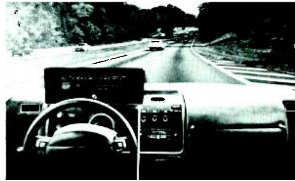
Fig. 7 Driver's view of the self-scanning display shows how above-the-dash location keeps driver's eyes close to the road while checking display information. Driver has choice of two display modes, with emergency messages overriding in case of a malfunction. Display is both digital and bar-graph in form.
