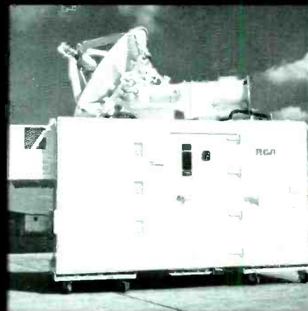
AN/TPQ-39(V) radar, a recent development designed specifically for the small, low-budget ranges known as the Digital Instrumentation Radar (DIR). It is one of the first radars to incorporate functional computer control.
