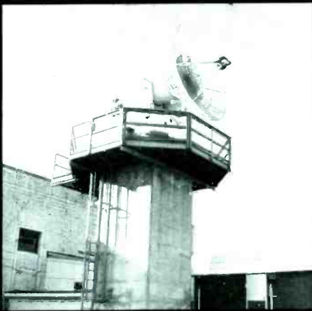
AN/FPS-16 radar installation at MSR, Moorestown. This unit is used as a test bed for system modifications in support of the world-wide range instrumentation network.
