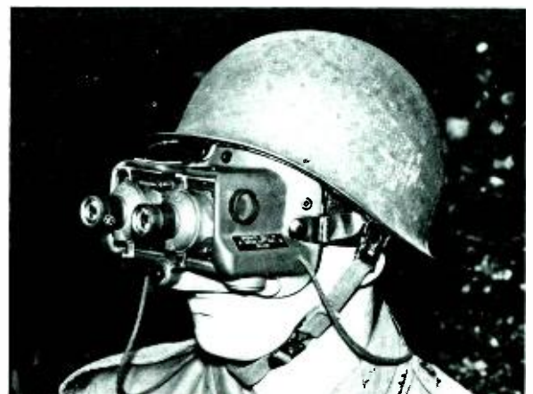
Fig. 1 Night vision goggles provide night-scene viewing under outdoor darkness with as little as starlight for illumination. RCA Electro-Optics and Devices in Lancaster manufactures image-intensifier tubes used in systems of this type.
