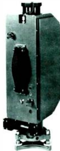
Fig. 6 Transmitter package contains all power converters and electronics except battery. Extra safety interlock prevents laser from transmitting unless it is aimed within seven degrees of vertical.
