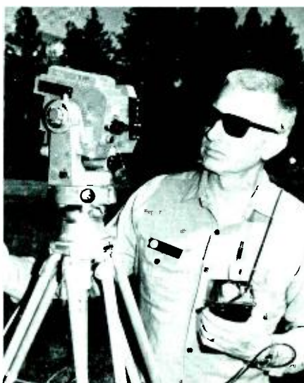
Fig. 2 Receiver theodolite subsystem is coarsely aimed at the transmitter's laser-light "pole" a mile or half-mile away, then adjusted in azimuth until the signal is acquired. Indicators tell which way to adjust aim until the receiver is aimed at the light pole within twelve arc-seconds.
