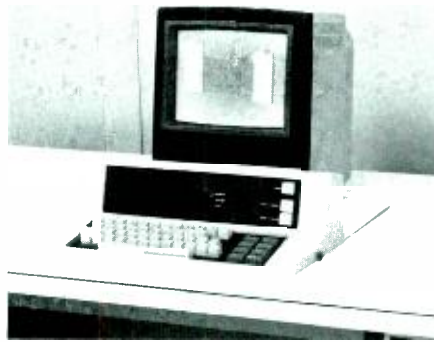
Fig. 5 Operator enters information into system via the composer. Editing can also be done here.
