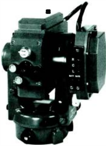
Fig. 5 Receiver resembles a standard theodolite. Indicators R, C, and L (for right, center, and left) tell which way to adjust receiver to center it on laser "pole."
