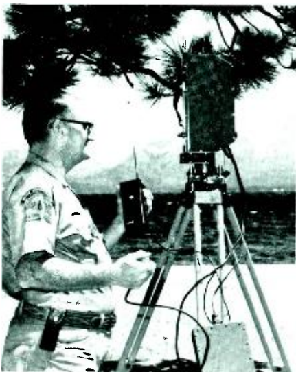
Fig. 1 Laser transmitter establishes a laser beam "range pole" rising a mile above reference point or boundary marker. Radio transceivers are used for voice communications and signaling between laser transmitter and receiver electronics.
