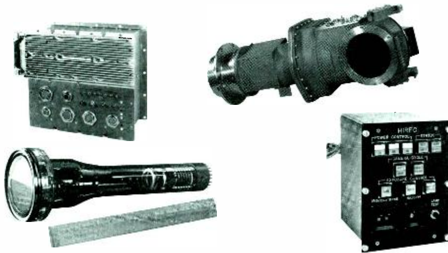
Fig. 3 Flyable camera components are grouped around the RBV tube (lower left), the heart of the electronic camera.
