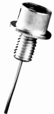
Size contrast: He-Cd gas laser and power supply (above); and GaAs solid-state injection laser, shown both unmounted (through the eye of a needle) and in final-product form.
