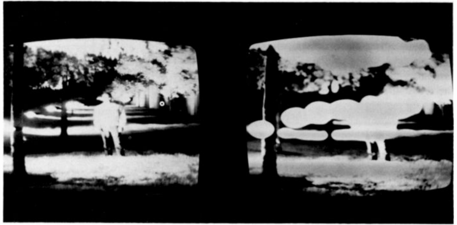
Fig. 9 Improved picture of a reduced-blooming silicon-target tube (left) compared with picture from a conventional silicon-target tube (right).
