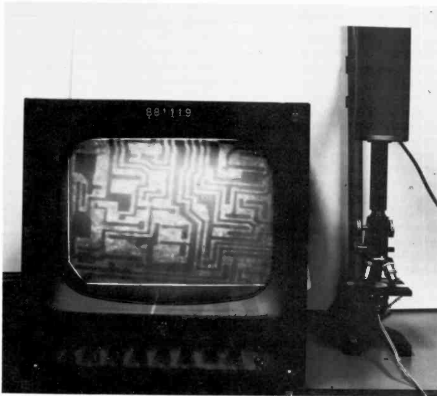
Fig. 12 Inspection application uses silicon vidicon's ir-sensitivity to "see" through silicon IC wafer.
